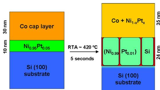
FIG. 1. (Color online) Schematic diagram illustrating the thin-film structure before and after RTA at 420 °C for 5 s. The color red indicates the GBs and shows the columnar nature of the  $(\text{Ni}_{0.99}\text{Pt}_{0.01})\text{Si}$  grains with the long axis oriented normal to the thin film's surface.
