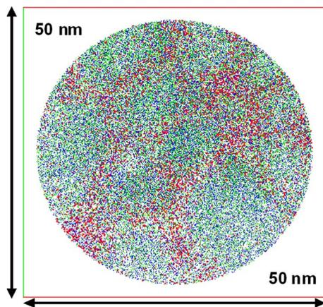
FIG. 2. (Color online) Two-dimensional (2D) top-view projection along the analysis direction of a full 3D reconstruction of 3D atom-probe tomographic data displaying the distribution of elements. Nickel, Si, and Pt atoms are shown in green, blue, and red, respectively. An analysis volume of  $50 \times 50 \times 5 \text{ nm}^3$  ( $4 \times 10^5$  atoms) is displayed from the silicide region of the complete reconstruction. Only 25% of the Ni and Si atoms are displayed for clarity.
